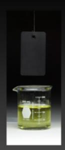
The ability of Cerakote™ H-146 to resist chemical attack was tested by dipping coated panels into a series of solvents to which the coating may be exposed during regular use and extreme conditions. The panels were placed in the solution and allowed to sit for 24 hours. Afterward, the samples were removed, analyzed and assigned a rank depending on the resistance to each specific chemical. The results of this test are shown in the table below.
